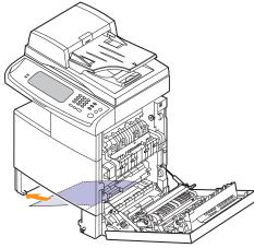
Once you remove the jammed paper here, open the side cover and then close it to clear the error message on the display.
